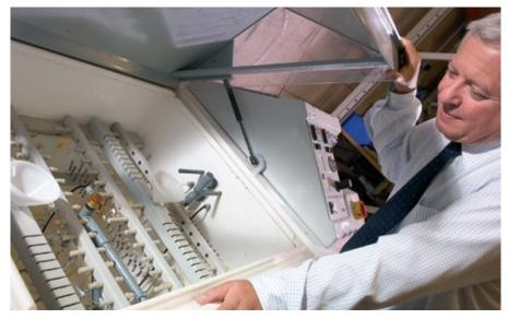
Using custom designed and built equipment, window screws are tested for speed of insertion, ensuring that self-drilling screws provide fast and efficient fastenings into steel reinforcement and that screws for fastening into PVC-U self-start easily and safely.
