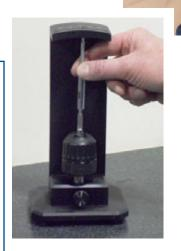
All aspects of our screws are tested and their dimensions checked to ensure that our high specifications are met. This includes depth of recess and 'wobble', using a certified Phillips No.2 driver bit. The internationally accepted standard is plus-orminus 6°.
