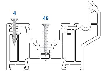
4 CFG 4.3 x 25 Z Hinge to main frame 5 CFG 4.3 x 30 Z Keeps to main frame
