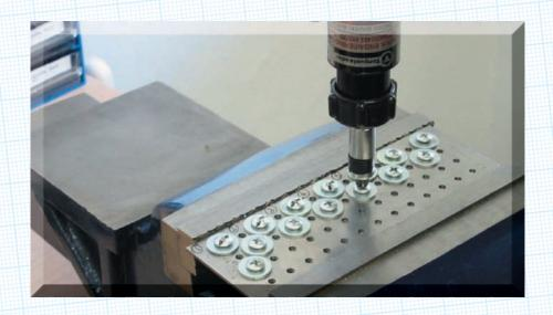
Every batch of *Rapierstar* screws is tested to ensure that optimal torsional strength and design specifications are met and exceeded.
