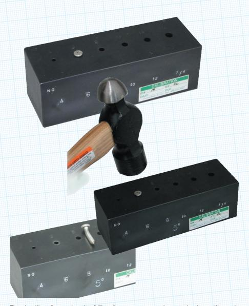
The ductility of every batch of **Rapierstar** screws is tested using calibrated test blocks, which have an angled upper surface conforming to acknowledged standards.
