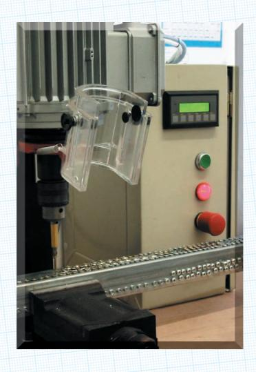
Using custom designed and built equipment, every batch of **Rapierstar** screws is tested to ensure that the speed of insertion meets Rapierstar's own high specification, resulting in faster, more cost effective production for you, the customer.
