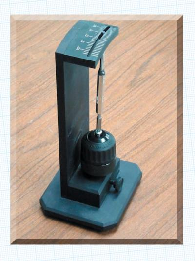
Each batch of **Rapierstar** screws is tested for "wobble" using a certified plug gauge. The international recommendation for this test allows 12° of movement. Rapierstar specify, and only accept 6° of movement, making insertion and fabrication easier and safer.
