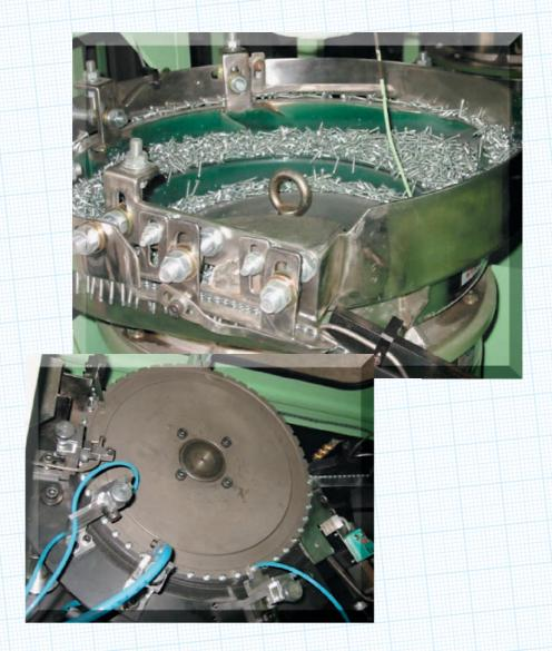
At the manufacturing stage, every batch of *Rapierstar* screws is laser sorted to check dimensions. During this process, swarf is also removed, which means that the finished boxes contain no foreign bodies. This means you are less likely to experience blockages where auto-feed machines are used.
