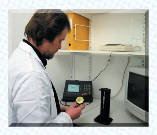
All dimensions are checked on every batch of *Rapierstar* screws, including the depth of the recess, which is measured using finely calibrated dial indicator gauges. The correct depth of recess means that the screwdriver bit fits perfectly, ensuring safety for your fabricator.
