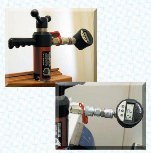
Pullout testing ensures that tensile strength and grip criteria are maintained.
